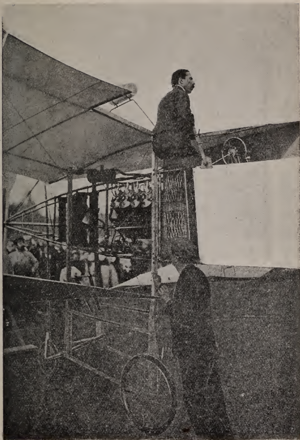
PLATE XVII.—The Santos Dumont Aeroplane "No. 14 bis." A View of the Engine, with M. Santos Dumont in the Car.
